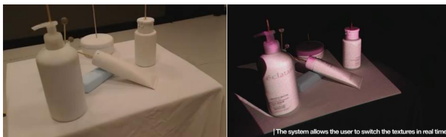
Figure 14: SAR example applied to industrial packaging design, pictures extracted from video [64]
