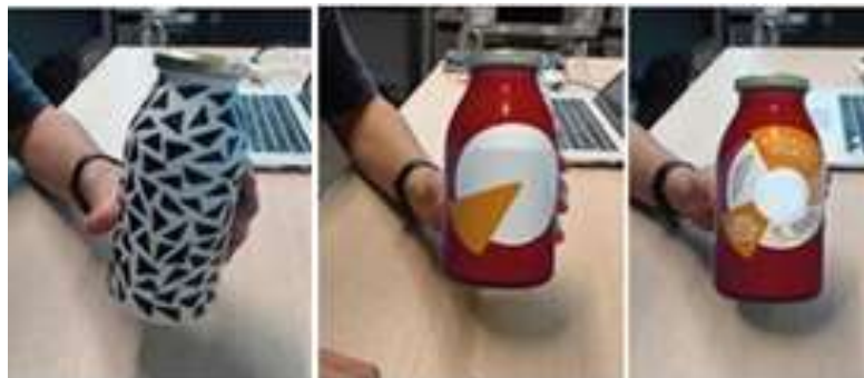
Figure 1: View of the Augmented Reality prototype i) without augmentation, showing the marker pattern ii) with augmentation - design in progress, iii) with augmentation - completed design proposal.
