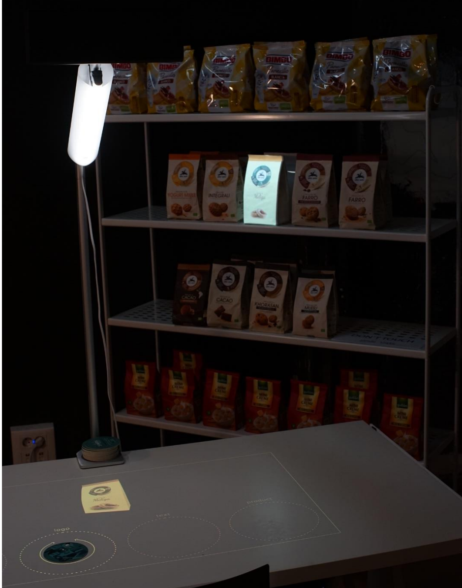
Figure 15 – Interaction with Concept Prototype T using a smart AR tangible tool. Note that, when viewed with the naked eye, the luminosity of the mixed reality pack appeared very similar to that of the real packs next to it.
